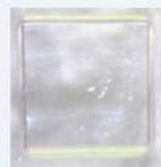
Electronic grade diamond containing single NV defects
